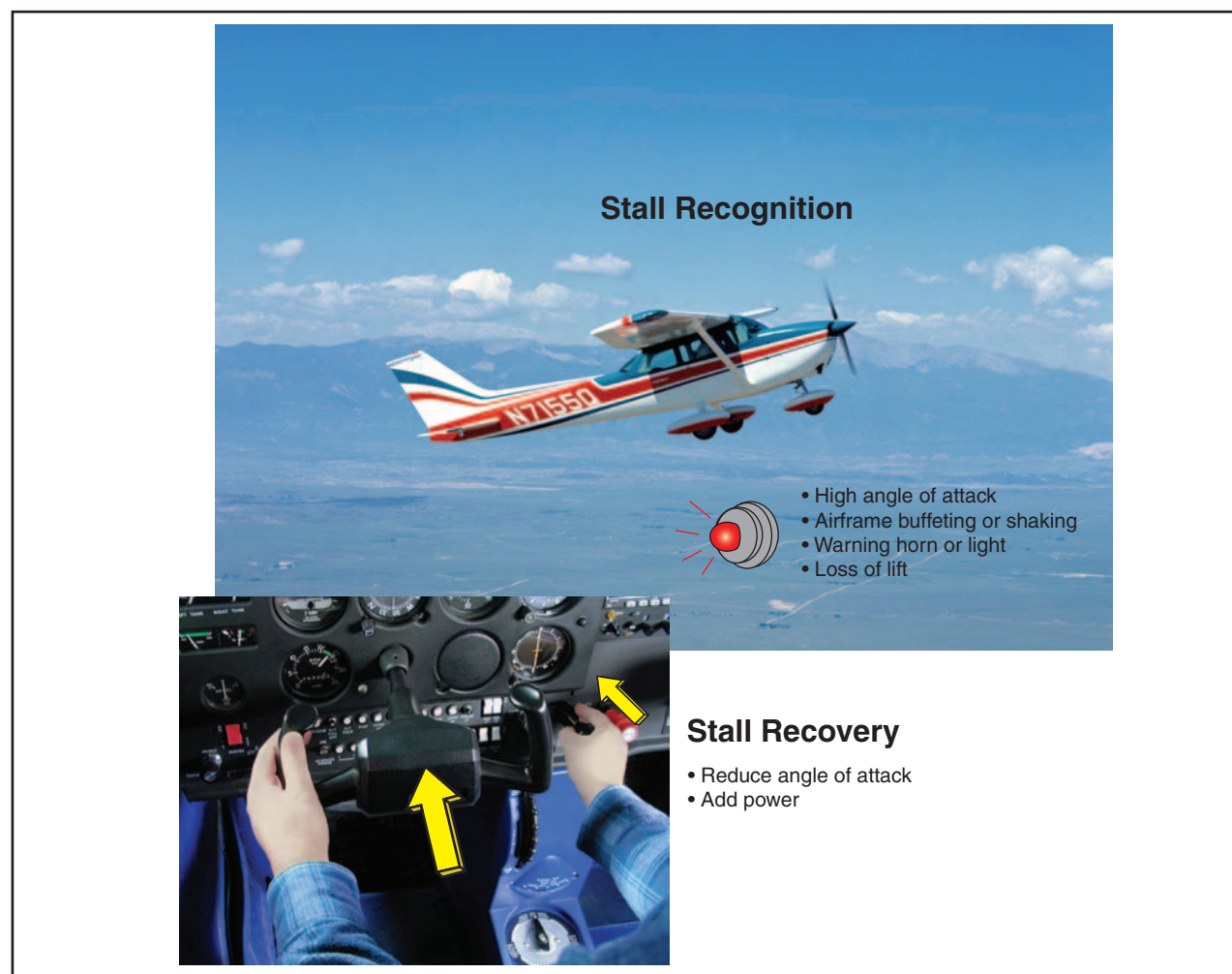
Figure 4-3. Stall recognition and recovery.
