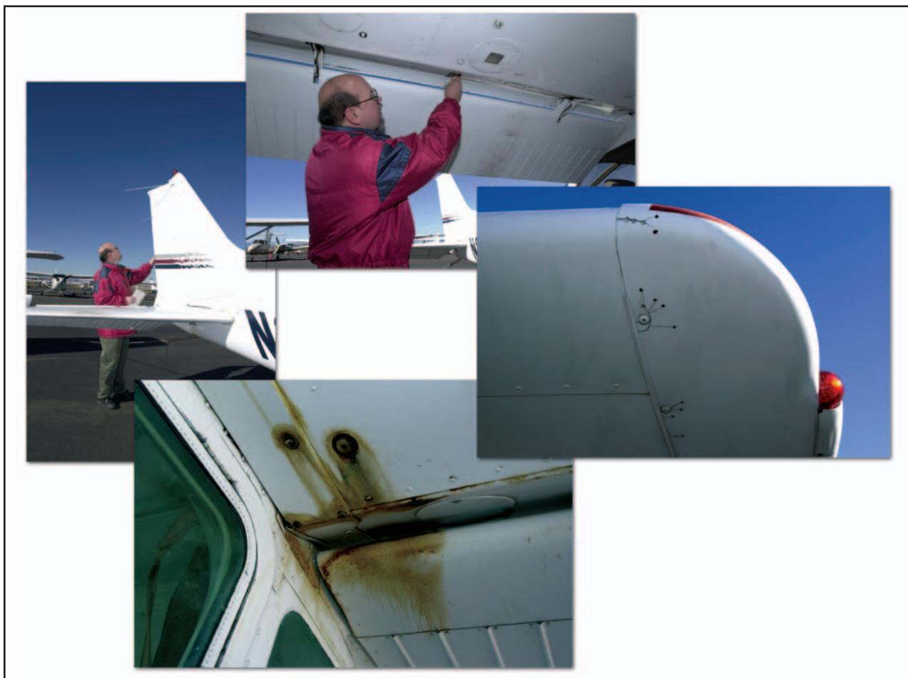
Figure 2-6. Wing and tail section inspection.
