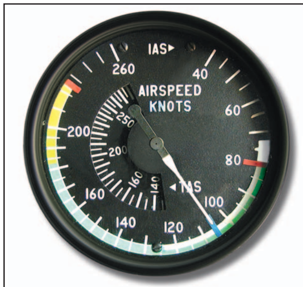
Figure 12-1. Airspeed indicator markings for a multiengine airplane.
