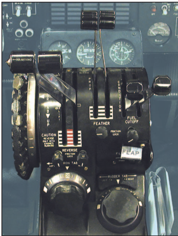
Figure 14-6. Powerplant controls—split shaft/free turbine engine.
