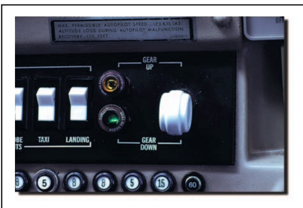
Figure 11-7. Typical landing gear switches and position indicators.
