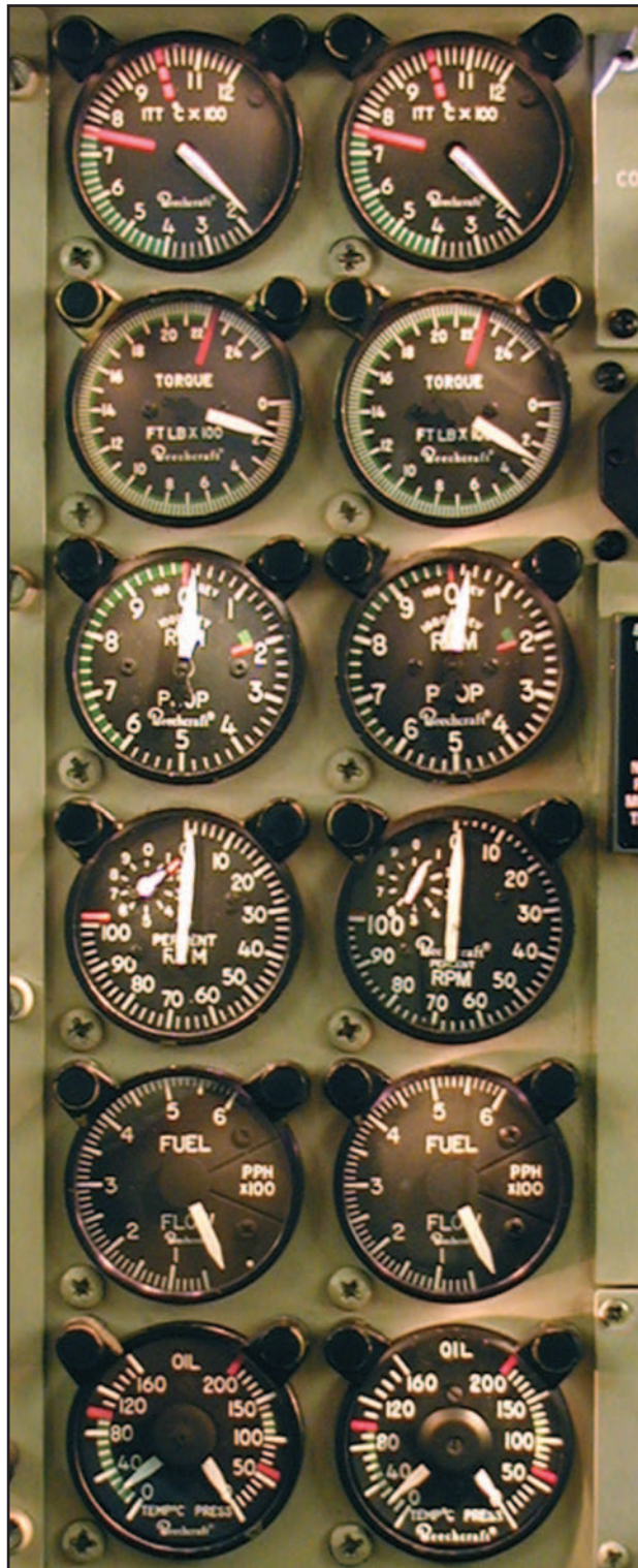
Figure 14-7. Engine instruments—split shaft/free turbine engine.
