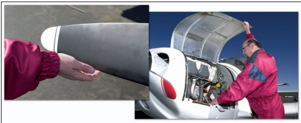
Figure 2-8. Check the propeller and inside the cowling.
